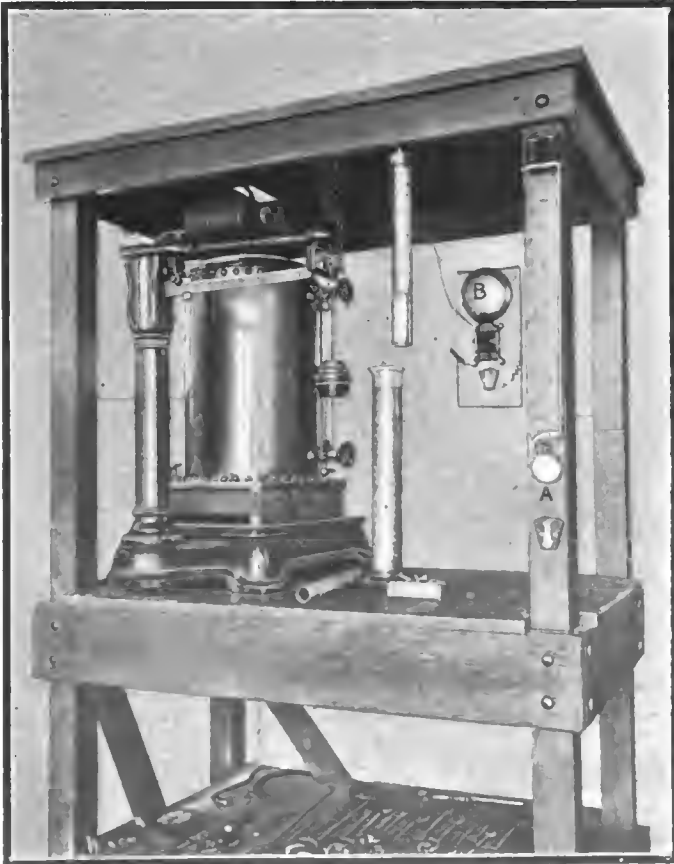
Fig. 2—Gasoline dispensing apparatus and scales with electrically operated stop watch attachment A, and bell B; feed pipe to carbureter not shown
